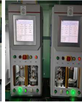
⑦Air tight test
